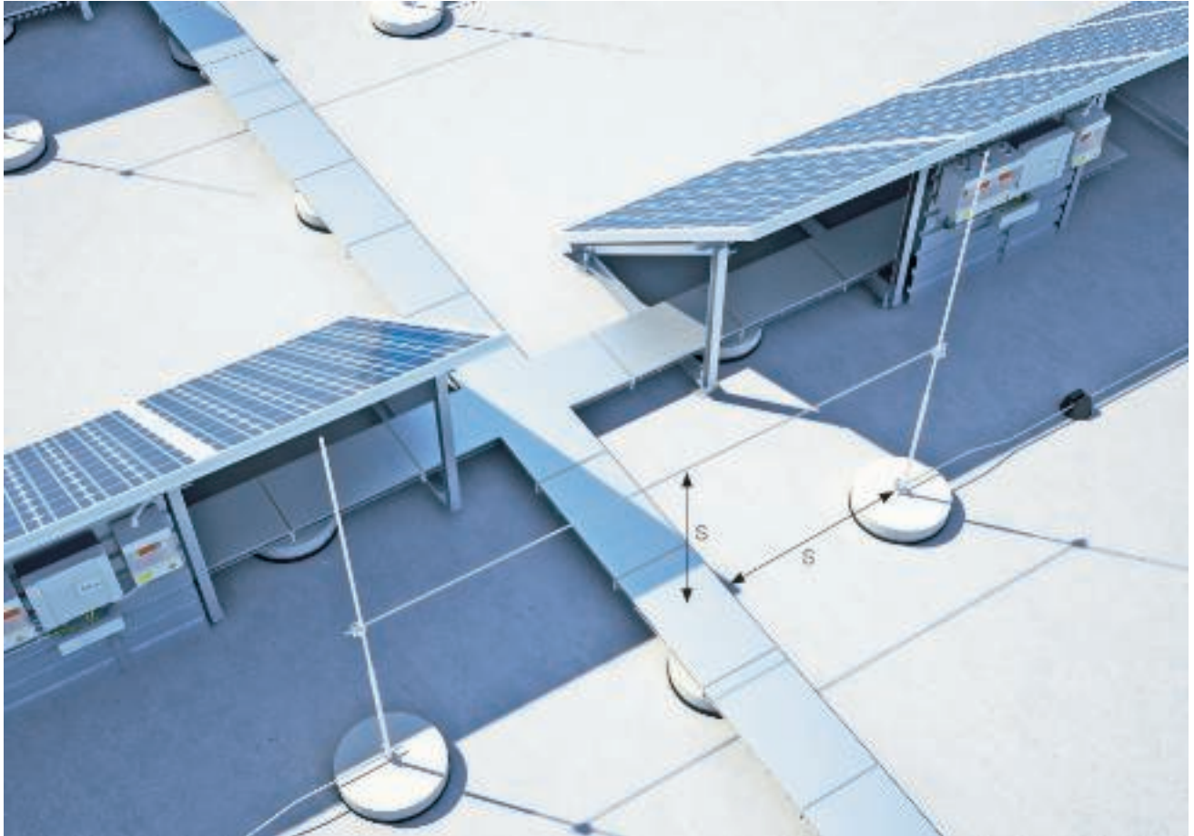
Figure 1: Separating distance (s) between the lightning protection system and cable support system
