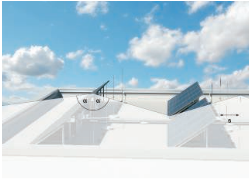
\alpha^\circ = lightning protection angle, s = separating distance
