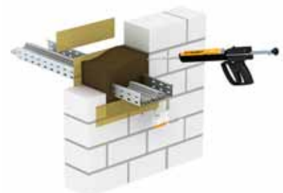
Insulation in a fire protection wall
