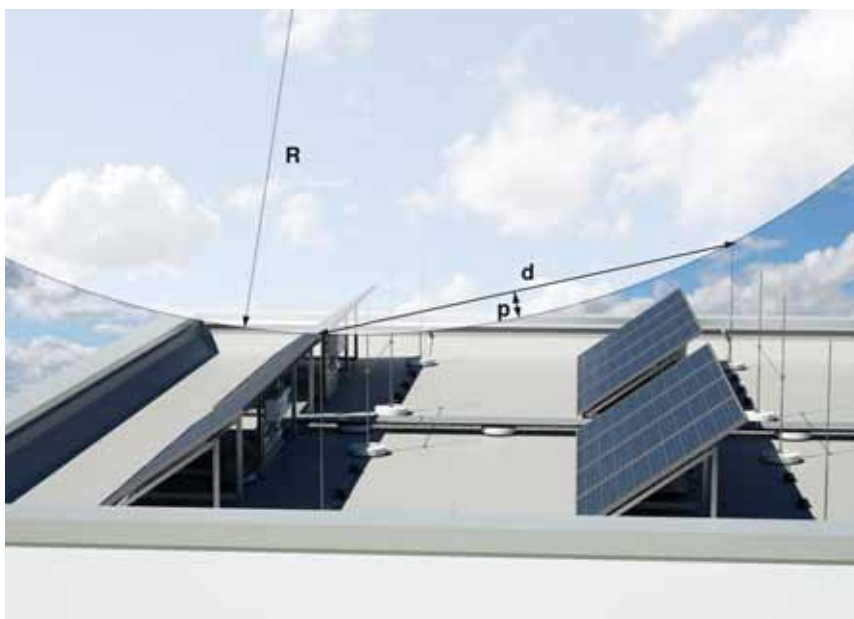
p = penetration depth, R = radius of the lightning sphere, d = distance of the interception system
