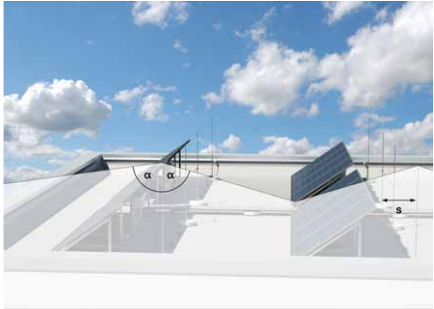
\alpha^\circ = lightning protection angle, s = separating distance
