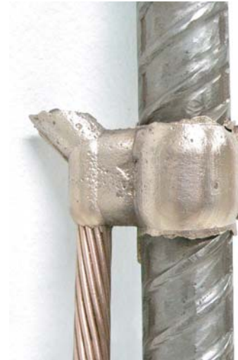
• 95 mm 2 Copper Cable to 40 mm Rebar
