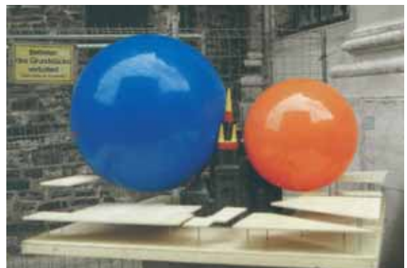
Fig. 5.1.1.6 Aachen Cathedral: Model with environment and “rolling spheres” for lightning protection systems Class II and III Ref.: Prof. Dr. A. Kern, Aachen
