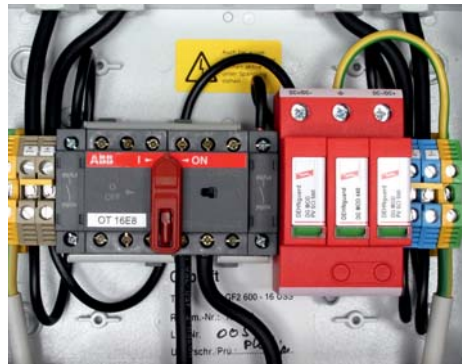
Fig. 9.18.1.2 Modular surge arrester Type 2 DEHNguard M YPV SCI FM with fault-resistant Y circuit and three-step d.c. switching element
