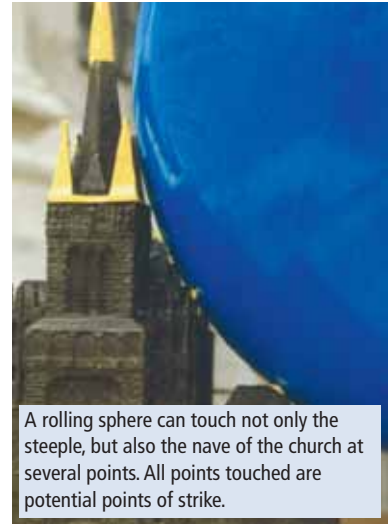
Fig. 5.1.1.2 Model of a rolling sphere Ref: Prof. Dr. A. Kern, Aachen
