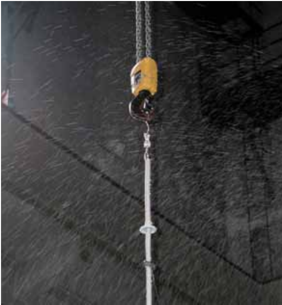
Fig. 5.7.1.3 Withstand voltage test under sprinkling
