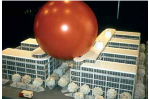
Fig. 5.1.1.4 Construction of a new administration building: Model with “rolling sphere” acc. to lightning protection system Type I Ref.: WBG Wiesinger
