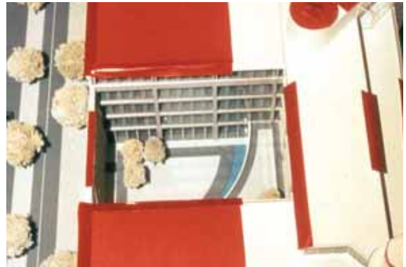
Fig. 5.1.1.5 Construction of a DAS administration building: Top view (excerpt) on the zones threatened by lightning strikes for lightning protection system Class I Ref.: WBG Wiesinger
