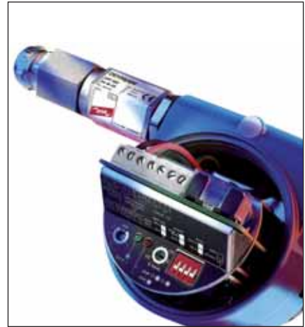
Fig. 9.3.13 Surge arrester DEHNpipe for outdoor areas for screwing into 2-wire process field devices
